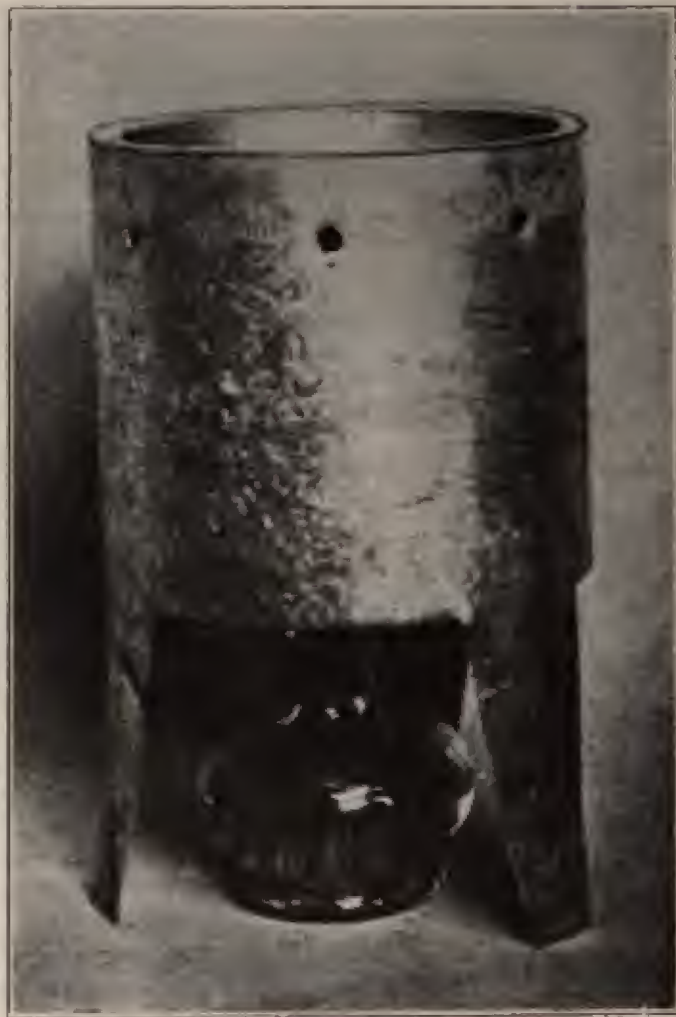
FIG. 30.— A simple apparatus for fumigating cellars, from piece of stove pipe.
